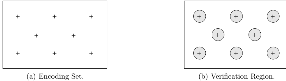
Figure 2. Encoding set and verification region for authentication watermarking. (a) All points marked with +’s form the encoding set \mathcal{C}(k) , which is a small subset of the signal space. (b) The shadowed area is verification region associated with key k . All codewords in the encoding set \mathcal{C}(k) and their legitimate neighbors are considered as authentic.
