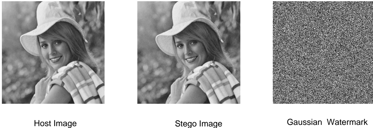
Figure 2. Example of steganography in a single image frame. (a) the host or cover-image frame, (b) the watermarked or stego-image frame, (c) the watermark containing the binary secret message.
